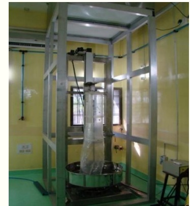
High pressure rinsing Set up
