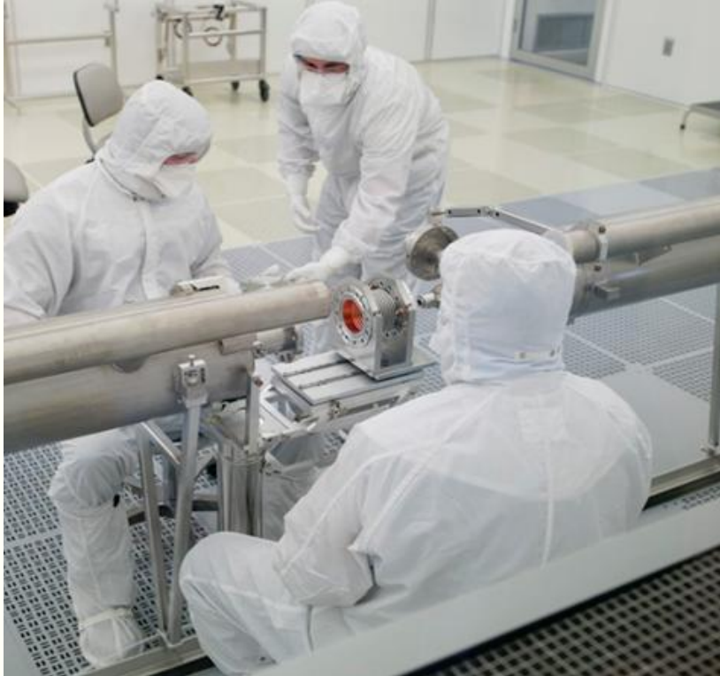
String Assembly in Class 10 area of MP9 Clean Room
