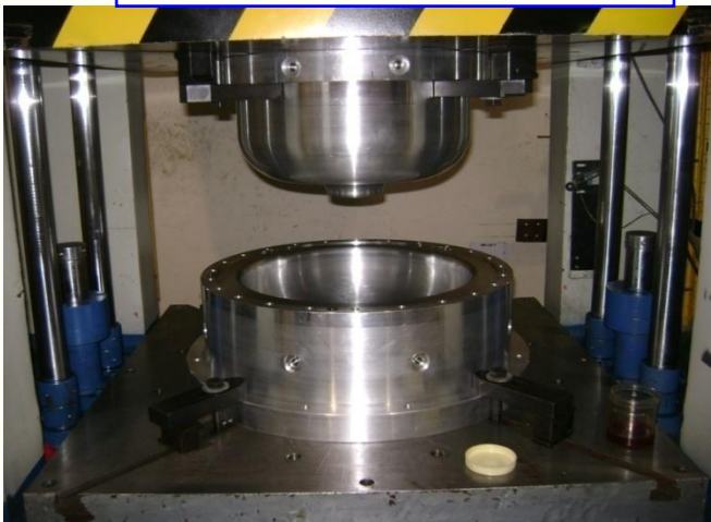
Die-Punch Set mounted on Press at RRCAT
