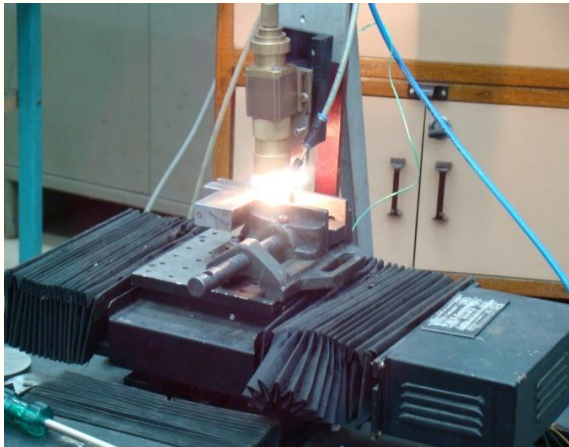
Laser welding of Cavity Support system at RRCAT
