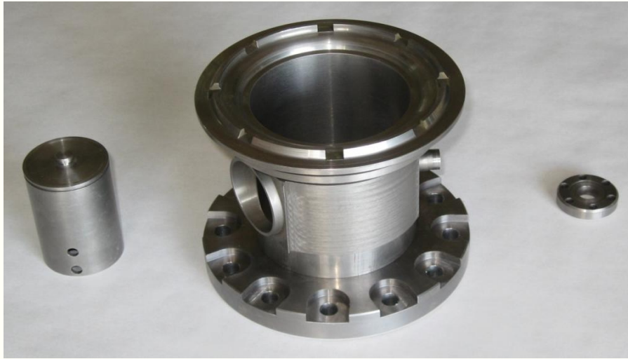
Development of prototype in Low RRR Nb completed at Workshop, RRCAT.
