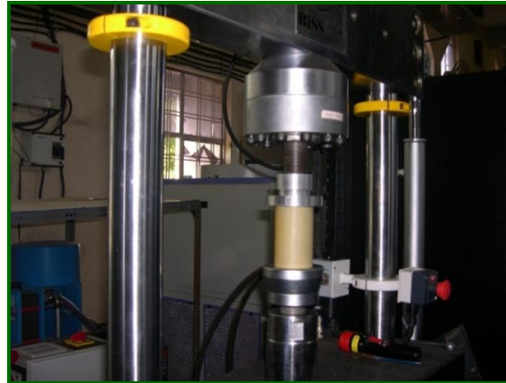
Load Testing of Cryogenic Support Post prototype at RRCAT
